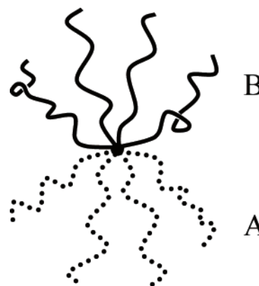
Figure 1. Illustration of an A_nB_n star block copolymer with n = 4 .
